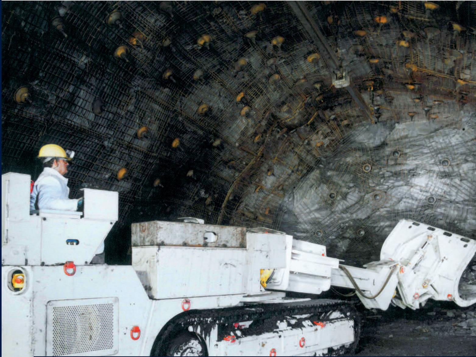
**HAZEMAG Side-dump Loader | HSL 2000**
